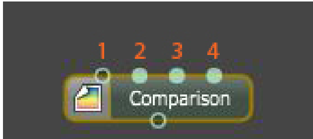
Figure 1: The various input pins for the Comparison node: (1) Input 1, (2) Input 2, (3) If A < B , (4) If A \geq B
